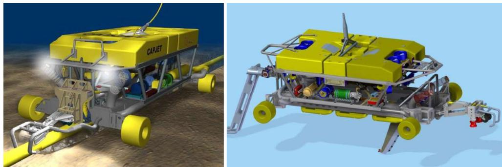
Figure 2.2 Capjet 1450 HP cable trencher (Nexans)
