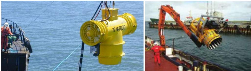
Figure 2.4 Examples of MFE (left: T4000 from James Fisher Subtech website, right: CCB-110 Excavator)
